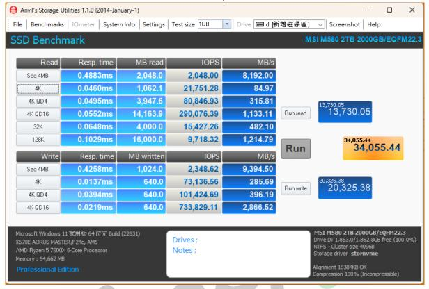
2.8.2 MSI M580 2TB PCIe 5.0 M.2 SSD performance with 50cm cable as below:
