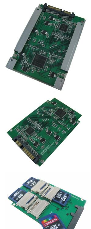
L914D is an economical 2.5" SSD. It uses a 2.5" ultra-lightweight aluminum material shell, coupled with the SD Card combination to SATA adapter. When assembled, it can operate in a variety of operating systems. Such as DOS, Windows 95, 98, XP, 2000, Vista, Win 7, Linux, Unix, and so on. L914D adapter allows the installation of SD Card as system disk, boot the operating system directly, without having to install any drivers.
