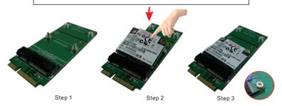
Step1: Put 2pcs of copper nuts on the holes for the half size mSATA SSD and fix with 2pcs of M2x6mm screws. Insert mSATA SSD into mini PCI-e socket.
