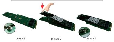
Step 1: Put copper nut on the same side of the NGFF connector; and fix M3x5mm screw from bottom to top of the adapter(picture 1).
