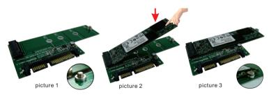
Step 1: Put copper nut on the same side of the NGFF connector; and fix M3x5mm screw from bottom to top of the adapter(picture 1).
