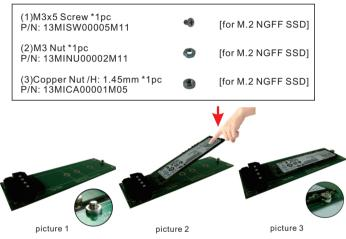
Step 1: Put copper nut on the same side of the NGFF connector; and fix M3x5mm screw from bottom to top of the adapter(picture 1).
